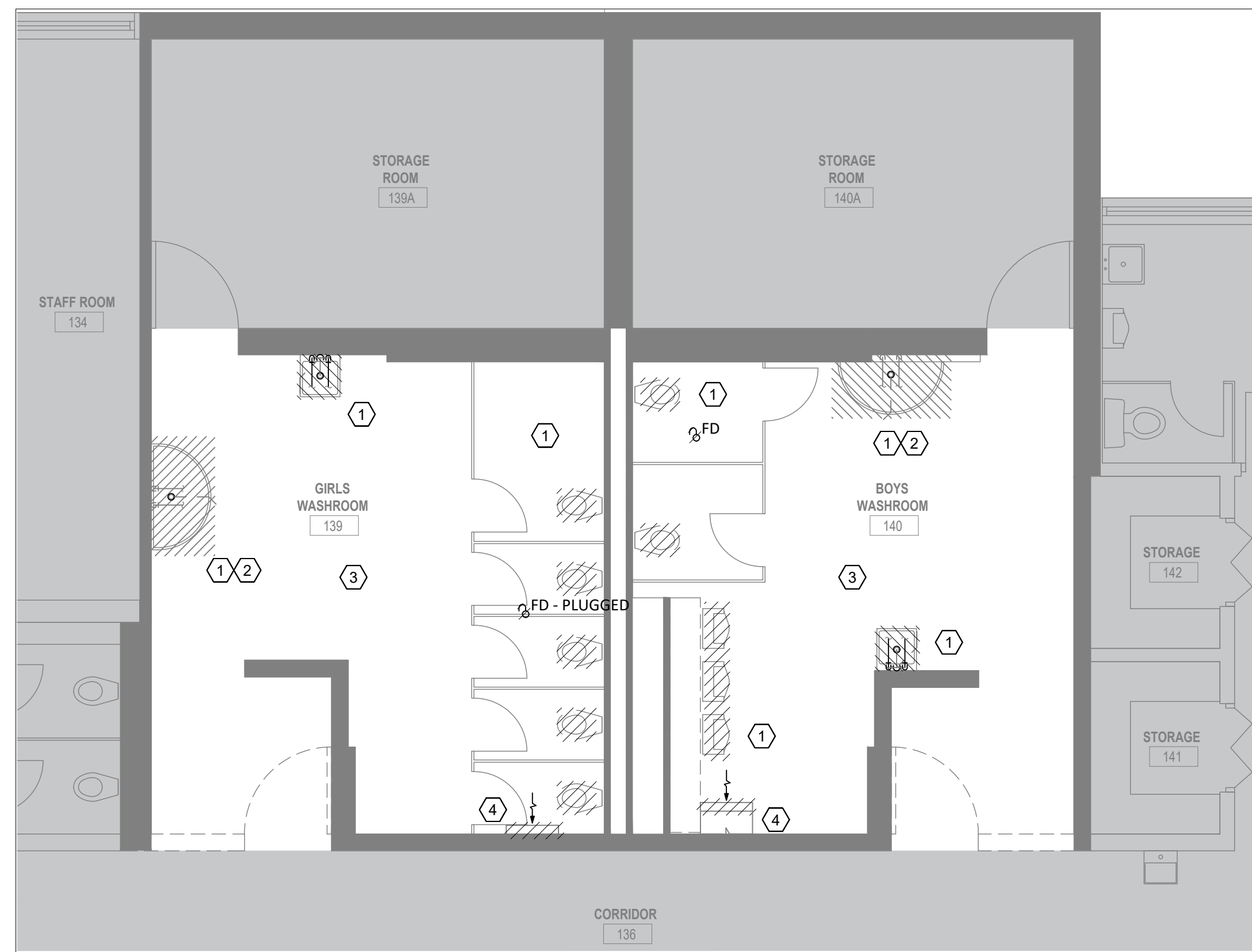
2 ROOMS 139, 140 MECHANICAL DEMOLITION - FULL RENOVATION M-1.01 1:50
