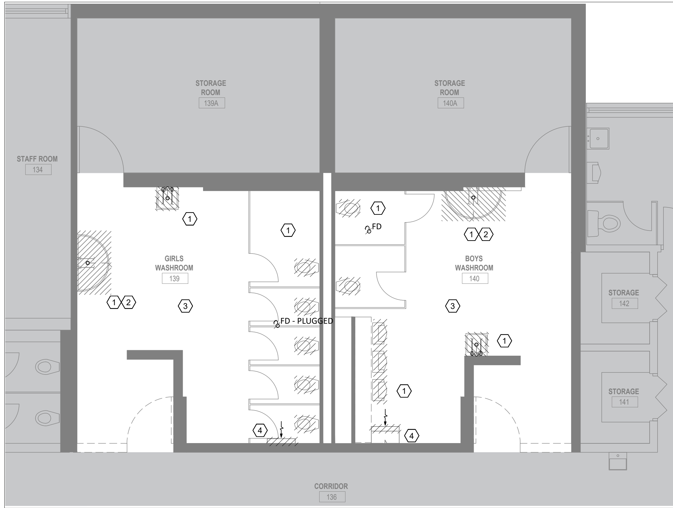
2 ROOMS 139, 140 MECHANICAL DEMOLITION - FULL RENOVATION M-1.01 1 : 50
