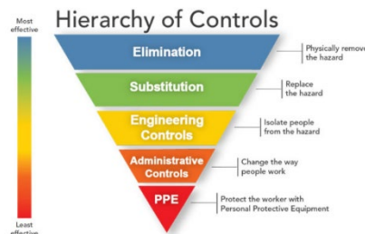
FIGURE 1 HIERARCHY OF CONTROLS [SOURCE: NIOSH]
